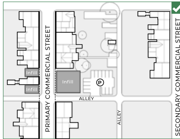
New infill development should be oriented to the street edge with parking located behind.
