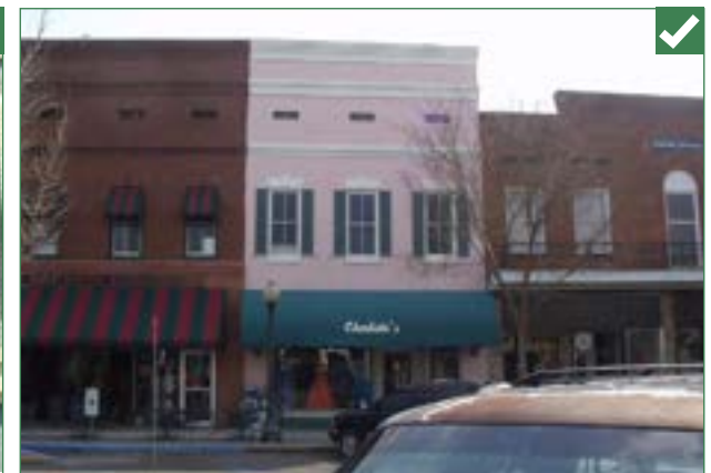
The horizontal alignment of windows unifies these three buildings of dissimilar heights, colors and detailing.
