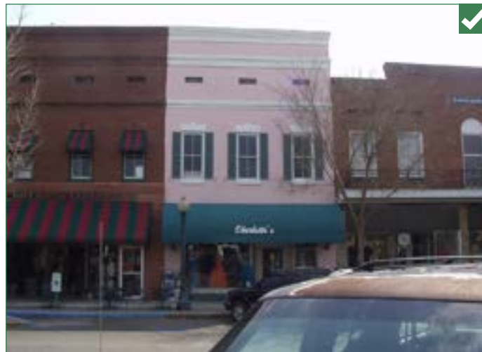
The consideration of horizontal alignment of door (storefront) and window elements in new building to the right unifies these three buildings of dissimilar heights, colors and detailing. Predominantly 2-over-2 window patterns used here.
